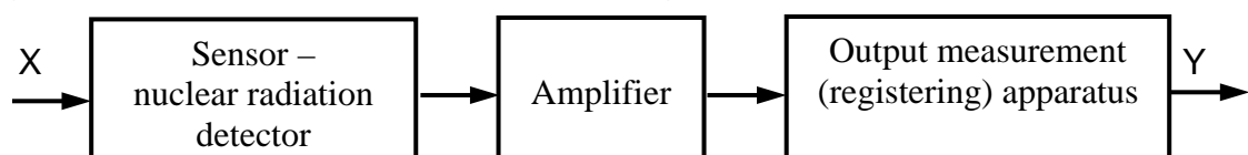
Fig.1. The general scheme of all dosimeters.
